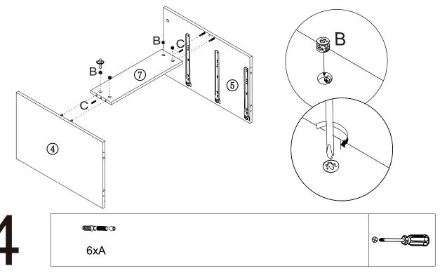
STEP 4: Fix cam pin (A) to panels(3)(5).
